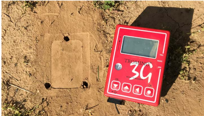
FIGURE 5. The MoHo Tromino® Tomograph in the field at an ideal site. The ground surface was cleared of any vegetation before positioning the Tromino® instrument.
