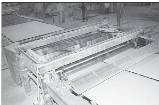
Conveyor system for making wallboard at the BPB-Celotex operation in Ottawa County. Photo by Michael D. Williams.
