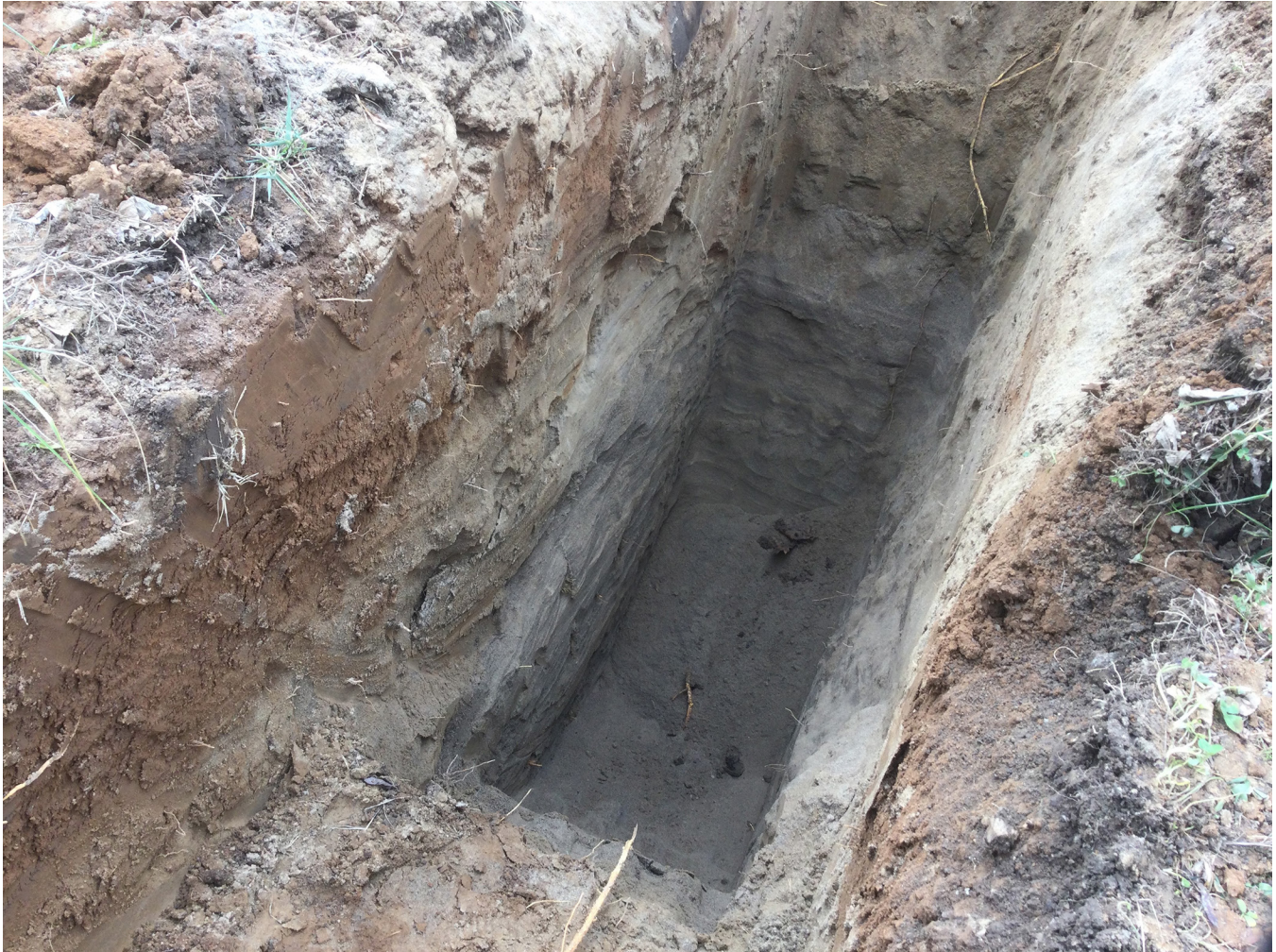
FIGURE 3-25. Photograph of pit dug to collect an OSL sample from the sands deposited at an alluvial fan at the mouth of the Washington Esker.
