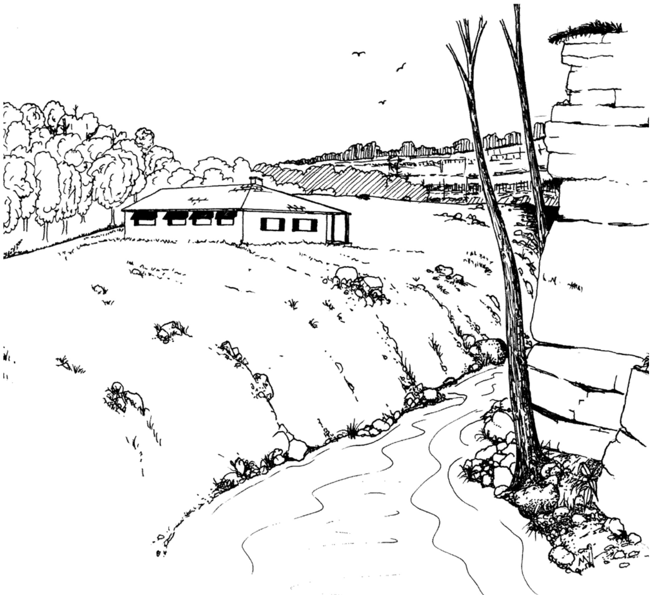
Home built on mine spoil next to dangerous highwall.
