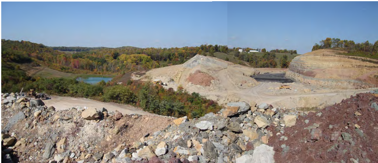
(ABOVE) Be-N Coal, Noble County, with active mining of an open coal pit (at right) and a sediment pond (at left).
