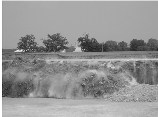
Detonation of explosives is a mining process to break and move rock materials.
