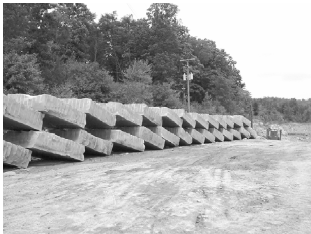
Large dimension stone will be cut into smaller pieces for a variety of building uses.
