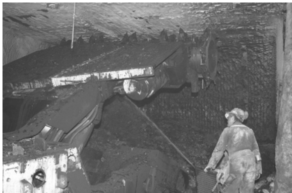
A continuous mining machine excavates coal in a room and pillar underground mine.
