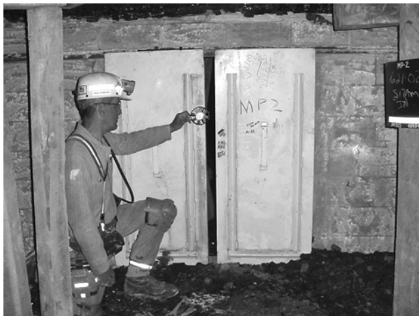
DMRM mine safety inspector checks air quality in an underground mine for oxygen and hazardous gases.
