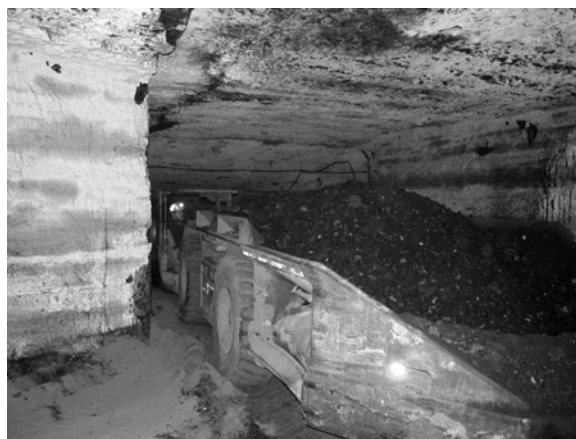
A coal shuttle car moves coal from a continuous mining machine to a conveyor belt that carries it to the surface.
