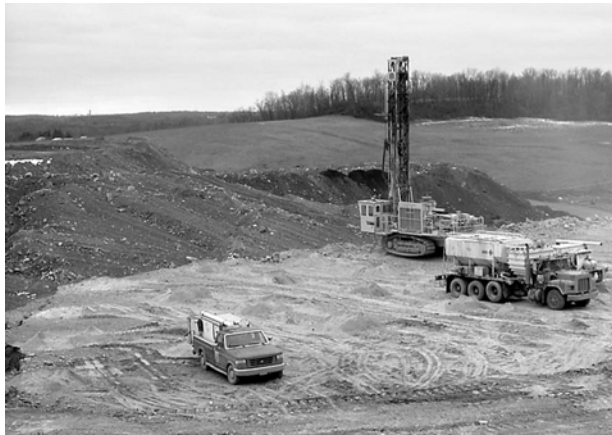
Holes are drilled and loaded with explosives in preparation for a blast.
