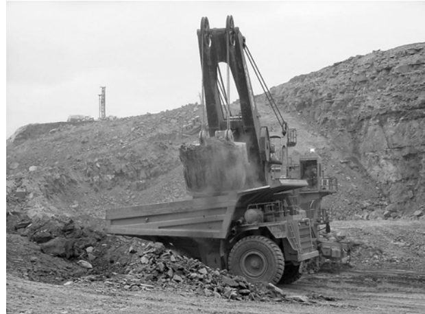
A haul truck is loaded with overburden, the soil and rock that lie above the desired coal seam.
