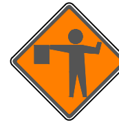
W20-7 COVER OR TURN DURING EVENINGS OR WHEN BOTH LANES ARE OPEN (500' FROM FLAGGER, BOTH SIDES OF ENTRANCE)
