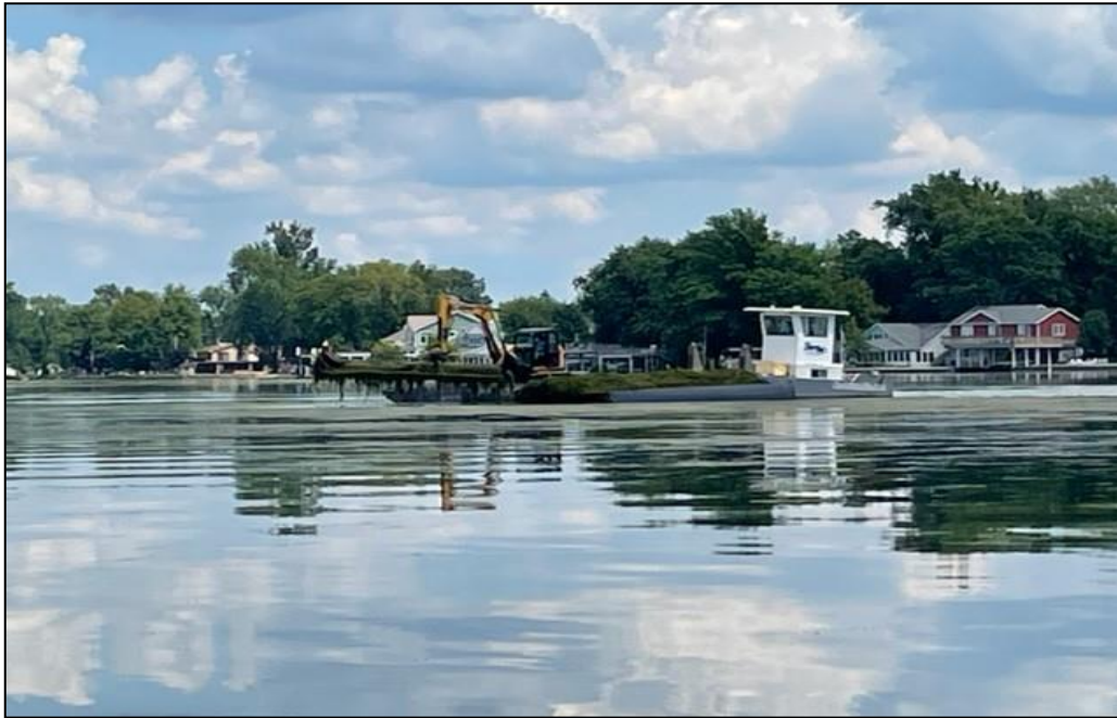
Figure 65. A mechanical harvester used to remove aquatic plants in Indian Lake (©RLS).
