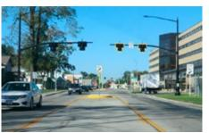
A pedestrian hybrid beacon (PHB) stops traffic so pedestrians can cross safely. The beacon, which is two red signals above a yellow one, is activated by pedestrians when they want to cross the street. First, yellow warning lights flash letting drivers know to slow down. Then there is a solid red light, telling drivers to stop so pedestrians can cross. When the beacon begins flashing red, drivers can proceed if the crosswalk is clear.
