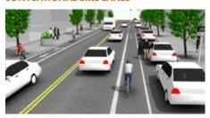
A conventional bike lane is located next to motor vehicle travel lanes and flows in the same direction as vehicle traffic. Bike lanes are typically on the right side of the street, between the adjacent travel lane and curb, road edge or parking lane.
