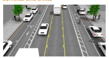
Buffered bike lanes are conventional bicycle lanes paired with a designated buffer space separating the bicycle lane from the adjacent motor vehicle travel lane and/or parking lane. Drivers must remember to yield to bicycles in the bike lane before turning across the lane.
