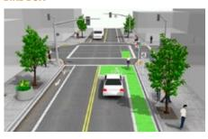
A bike box is a designated area at the head of a traffic lane at a signalized intersection. It provides bicyclists with a safe and visible way to get ahead of queuing traffic while the light is red. A bike box also helps bicyclists turn left safely and can prevent "right hook" conflicts when vehicles are turning at an intersection.
