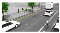
Contra-flow bicycle lanes are bicycle lanes designed to allow bicyclists to ride in the opposite direction of motor vehicle traffic. Contra-flow lanes are separated with yellow center lane striping.
