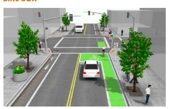
A bike box is a designated area at the head of a traffic lane at a signalized intersection. It provides bicyclists with a safe and visible way to get ahead of queuing traffic while the light is red. A bike box also helps bicyclists turn left safely and can prevent "right hook" conflicts when vehicles are turning at an intersection.
