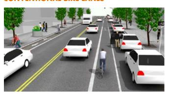
A conventional bike lane is located next to motor vehicle travel lanes and flows in the same direction as vehicle traffic. Bike lanes are typically on the right side of the street, between the adjacent travel lane and curb, road edge or parking lane.
