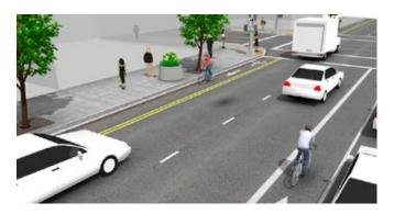
Contra-flow bicycle lanes are bicycle lanes designed to allow bicyclists to ride in the opposite direction of motor vehicle traffic. Contra-flow lanes are separated with yellow center lane striping.
