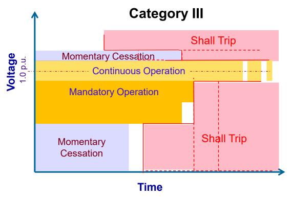
Dashed lines indicate permissible range of trip adjustment, solid lines indicate default settings.
