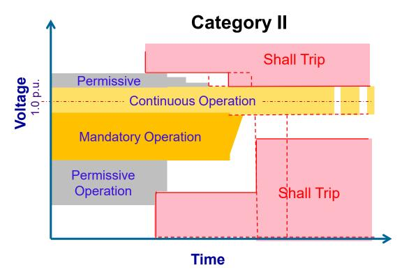
Dashed lines indicate permissible range of trip adjustment, solid lines indicate default settings.
