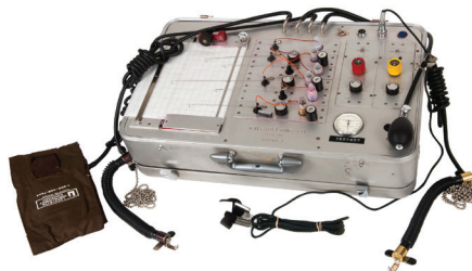
Left: The 1970 Stoelting Polygraph Instrument, which took approximately 30 minutes to warm up before use. It provided a continuous recording of blood pressure, heart rate, pulse, respiration and electrical skin resistance.
