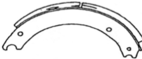
Out-of-Service Cracks or voids that exceed 1/16" in width. Cracks that exceed 1-1/2" in length.
