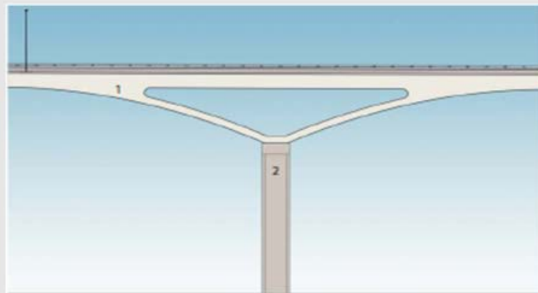
MAIN SPAN PIER SIDE ELEVATION (PIERS 3-11)
