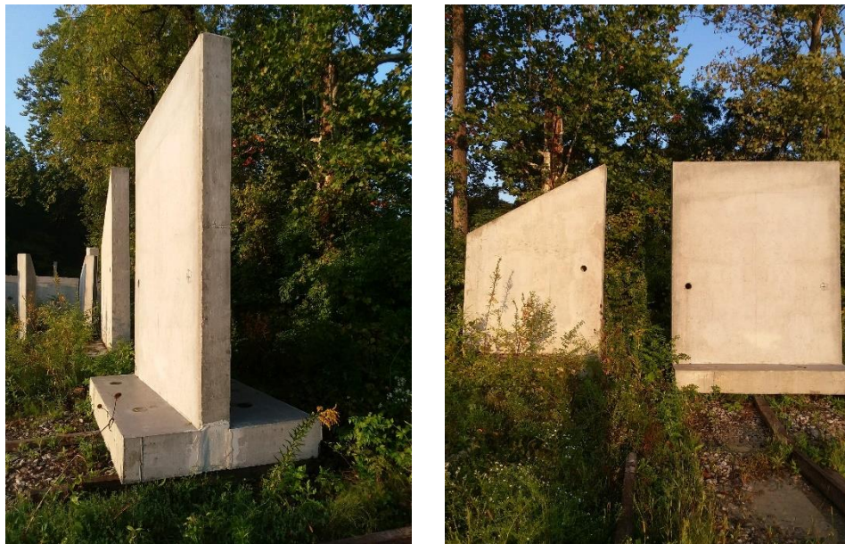
Figure 3: Completed Wingwalls at Mack Industries Before Shipment
