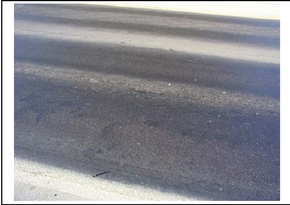
Photo E-3. Bleeding in Local Pavement, Medium Severity
