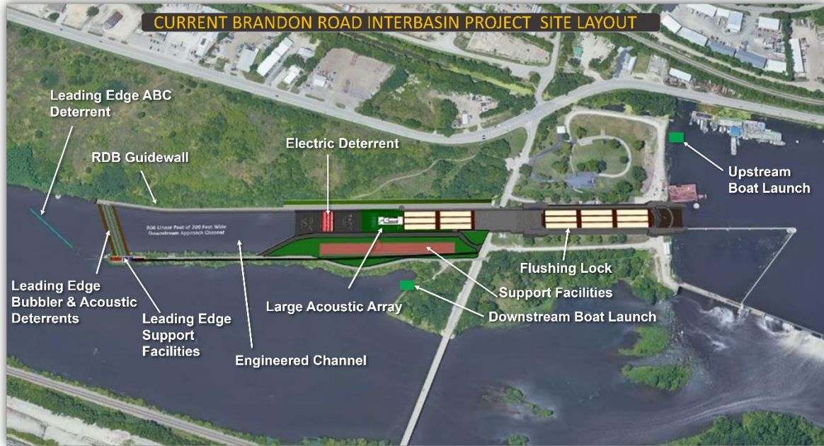
Figure 5: Brandon Road Lock and Dam AIS Counter Measures
