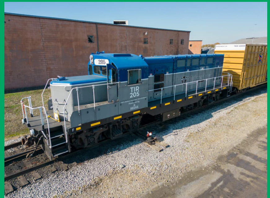
All-Electric Switcher Locomotive
