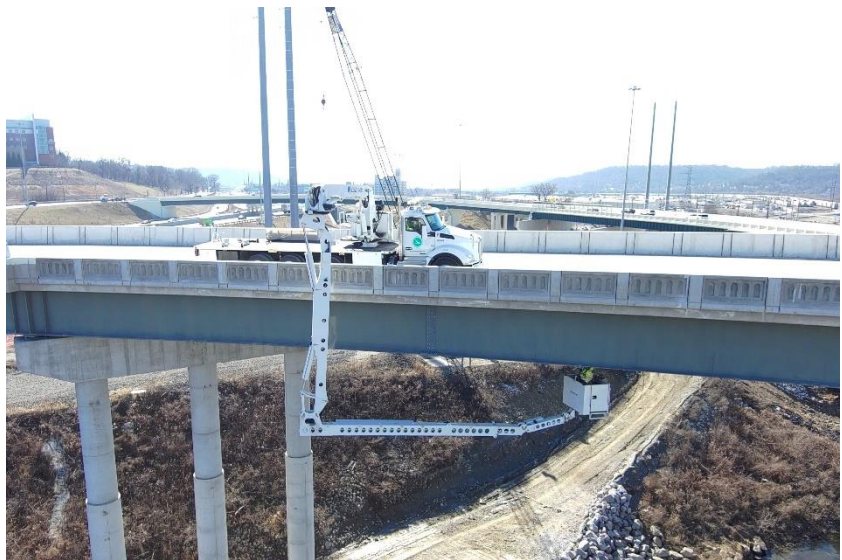
Figure 320 - Snooper Bucket Deployed for Right-Side Operation
