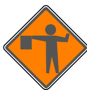
W20-7 COVER OR TURN DURING EVENINGS OR WHEN BOTH LANES ARE OPEN (500' FROM FLAGGER, BOTH SIDES OF ENTRANCE)
