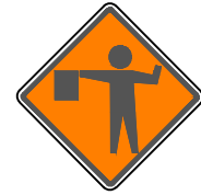
W20-7 COVER OR TURN DURING EVENINGS OR WHEN BOTH LANES ARE OPEN (500' FROM FLAGGER, BOTH SIDES OF ENTRANCE)
