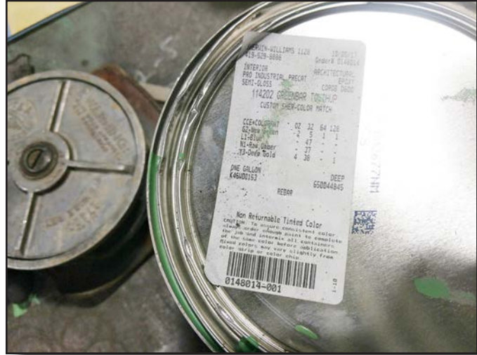
Lid showing epoxy paint not in compliance for use with Greenbar on ODOT projects.
